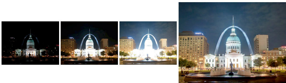
Figure 1: Example of three input images with different exposure levels and the resulting HDR image. Images from http://en.wikipedia.org/High_dynamic_range_imaging
